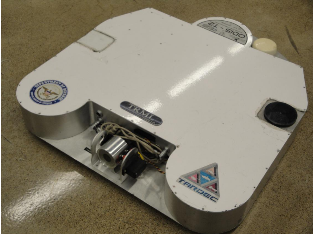
Figure 3: Front view of ODIS, Omni-Directional Inspection System.
