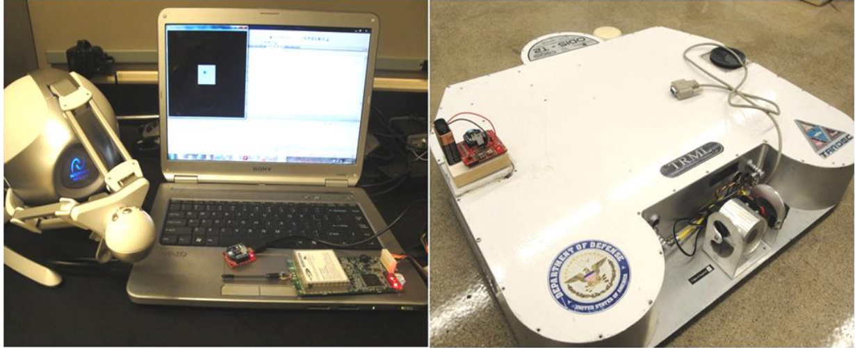
Figure 22: Absolute teleoperation system in the CARES lab. Left side showing the server with the Falcon haptic device, Xbee server module and Freewave radio attached and right side shows the ODIS robot with Xbee accelerometer on the top.
